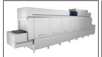
520128 (EFTD108EL2U3D1M5ER385) Flight Type Dishwasher, 4 tanks, 10800 dishes/h, electric, 950mm loading, 1600mm unloading, 1 dryer, 55mm conveyor, ESD, right to left
